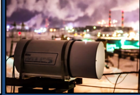
MTP-5 microwave temperature profiler (Norilsk only)
