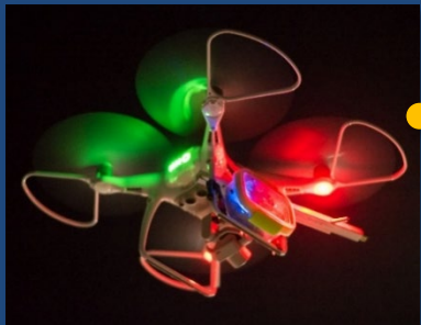
Quadcopter-based vertical temperature sounding over the city
