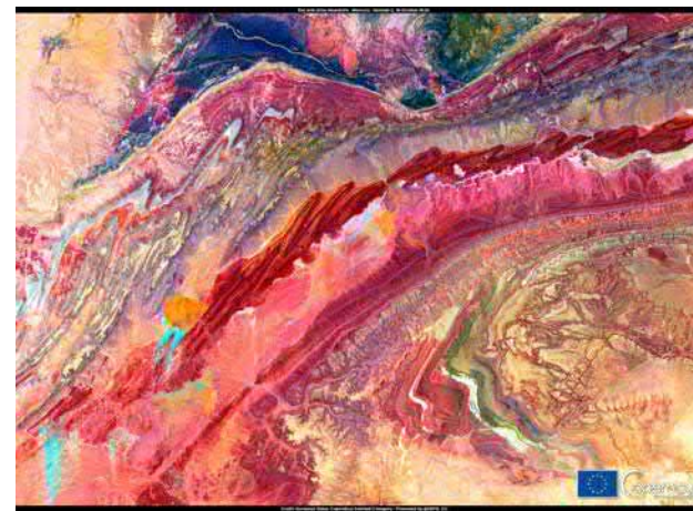
false-colour image, combining several bands of the multispectral imager to highlight the different rock types in the Anti-Atlas Mountains
